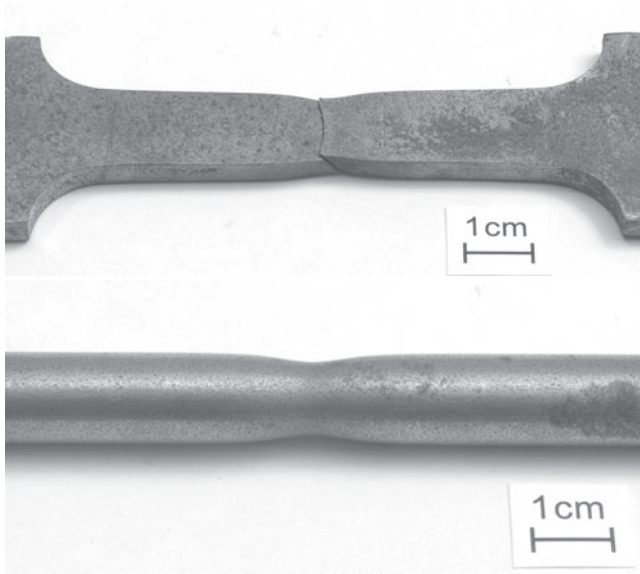
Figure 1.6. Examples of localization of deformation occurring for tensile loads in low-carbon steel samples. Top : Necking is the first mode occurring in the dog-bone-shaped strip shown in the figure. Later, shear banding (with a 45° inclination) develops within the necked zone, which eventually degenerates into a fracture (visible in the photo). Bottom : Necking in a cylindrical bar under tension.
