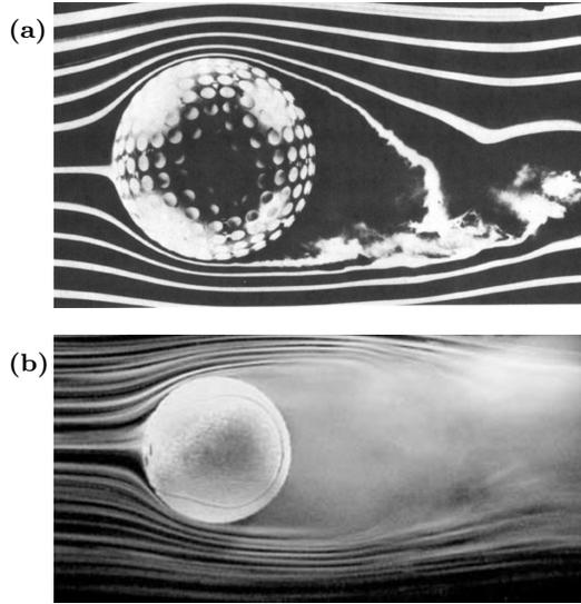
**Figure 1.2** Air flow around an object can be visualized using smoke. The flow around a golf ball is shown in (a) (Brown [1971]), and around a tennis ball in (b) (Bluck [2000]). In both cases the air is moving from left to right.
