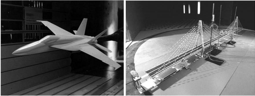
**Figure 1.4** Scale model testing. Dimensional analysis is used in the development of scale models used in wind tunnels. On the left there is a flight test of an F-18 model in NASA’s 11 ft transonic wind tunnel (NASA [2008]), and on the right a wind tunnel test of a 1:160 scale model of the Owensboro Bridge (Hsu [2009]).
