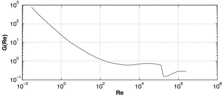
**Figure 1.3** The measured values of the function  $G(Re)$  that arises in the formula for the drag on a sphere, as given in (1.19).
