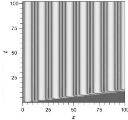
**Figure 1.7** Spatial pattern created in a plug-flow reactor (Bamforth et al. [2000]). The tube occupies the interval  $0 \leq x \leq 100$ , and starting at  $t = 0$  the chemicals are poured into the left end. As they flow along the tube a striped pattern develops.
