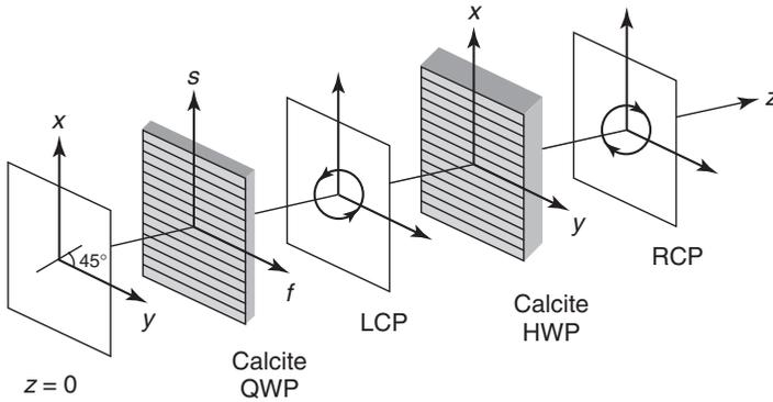
**Figure 1.10** A linearly polarized beam making an angle  $45^\circ$  with the  $x$ -axis gets converted to an LCP after propagating through a calcite QWP; further, an LCP gets converted to a RCP after propagating through a calcite HWP. The optic axis in the QWP and HWP is along the  $y$ -direction as shown by lines parallel to the  $y$ -axis. Light polarized along the  $y$ -axis travels faster than light polarized along the  $x$ -axis; hence the symbols  $f$  (fast) and  $s$  (slow).
