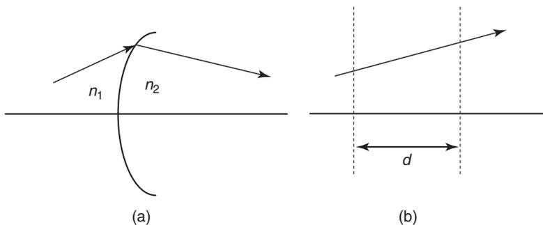
**Figure 1.3** (a) Shows a ray refracting at an interface between two media of refractive indices  $n_1$  and  $n_2$ . (b) A ray propagating through homogeneous medium.
