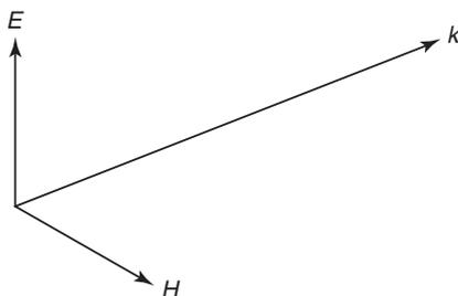
**Figure 1.1** A plane wave propagating along a direction specified by  $\mathbf{k}$ . The electric and magnetic fields associated with the wave are at right angles to the direction of propagation.
