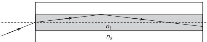
**Figure 1.11** An optical fiber consists of a core of refractive index  $n_1$  surrounded by a cladding of refractive index  $n_2$ .
