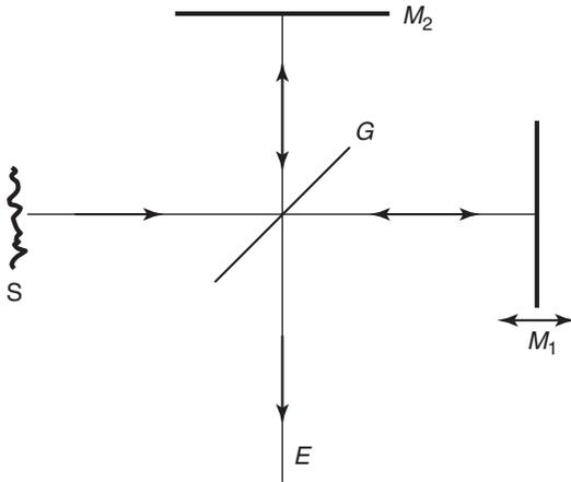
**Figure 1.8** Michelson interferometer arrangement.
