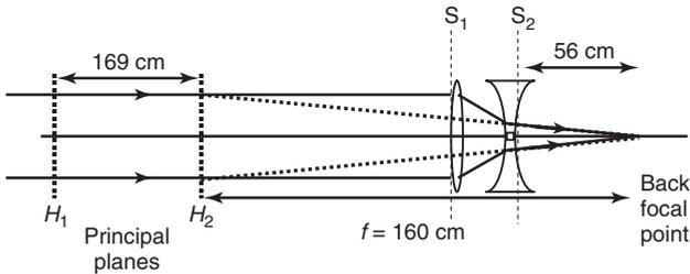
**Figure 1.5** An optical system consisting of a double convex and a double concave lens.  $H_1$  and  $H_2$  are the principal planes.
