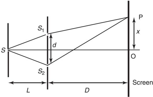
**Figure 1.6** Young's double-slit experiment. Light from a source  $S$  illuminates the pair of slits  $S_1$  and  $S_2$ . Light waves emanating from  $S_1$  and  $S_2$  interfere on the screen to produce an interference pattern.
