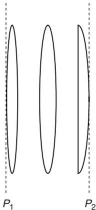
**Figure 1.4** An optical system formed by three lenses. The system matrix describes the matrix of propagation of the ray from plane  $P_1$  to plane  $P_2$ .
