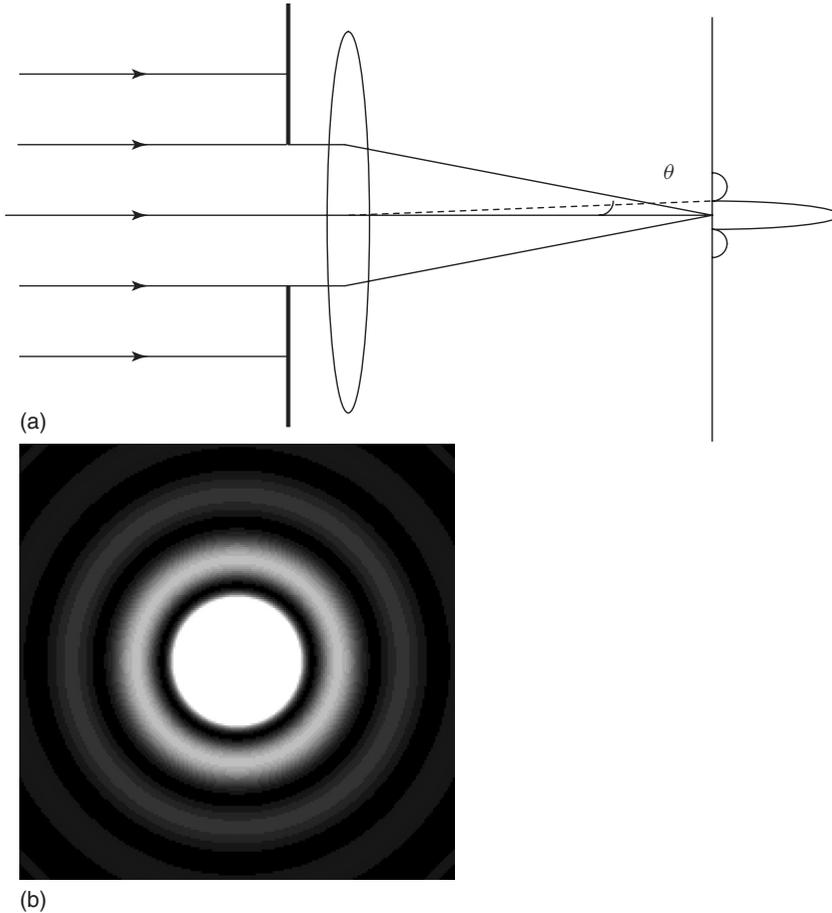
**Figure 1.9** (a) A plane wave falling on a circular aperture and forming an Airy pattern on the focal plane of the lens. (b) Airy pattern that will be observed on the back focal plane of the lens.
