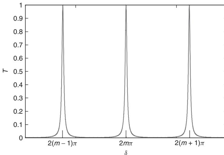
**Figure 1.7** The transmittance of a Fabry–Perot interferometer. The maxima of transmission correspond to integral multiples of  $2\pi$ . The higher the reflectivity of the mirrors the sharper would be the peaks.
