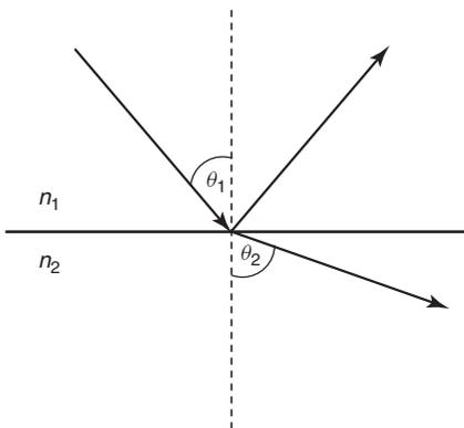
**Figure 1.2** A plane wave incident on a dielectric interface generates a reflected and a transmitted wave.
