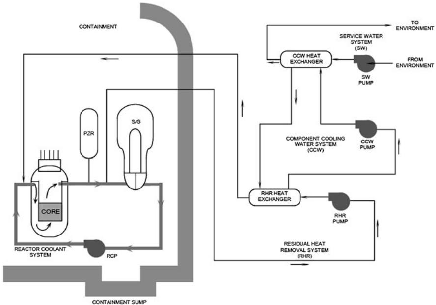
**Fig. 2.9** Schematic of RHR system and its major components ([www.nrc.gov/reading-rm/basic-ref/teachers](http://www.nrc.gov/reading-rm/basic-ref/teachers))
