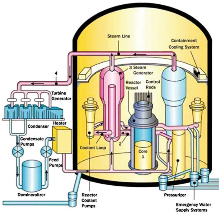
Fig. 2.2 Simplified PWR plant layout showing the major components of the containment building ([www.nrc.gov/reactors/pwrs](http://www.nrc.gov/reactors/pwrs))
