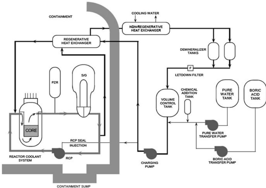
**Fig. 2.8** Schematic of CVCS system and its major components ([www.nrc.gov/reading-rm/basic-ref/teachers](http://www.nrc.gov/reading-rm/basic-ref/teachers))
