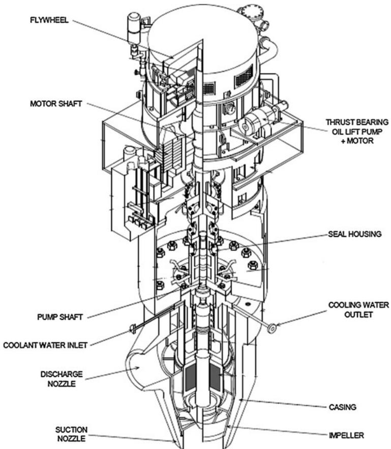
**Fig. 2.6** A reactor coolant pump and its major components (adopted from [www.nrc.gov/reading-rm/basic-ref/teachers](http://www.nrc.gov/reading-rm/basic-ref/teachers))
