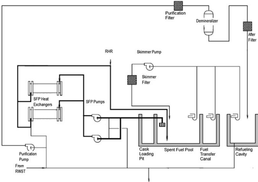
**Fig. 2.11** Schematic of spent fuel pool cooling and filtration and reactor cavity filtration systems (adopted from [www.nrc.gov](http://www.nrc.gov))
