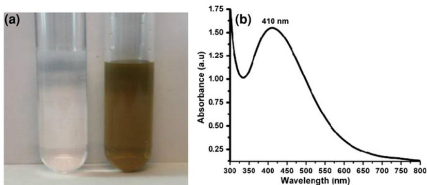
**Fig. 2.2** **a** Image of the test tubes containing  $\text{AgNO}_3$  solution before (test tube on the *left*) and after (test tube on the *right*) the formation of silver nanoparticles by the *S. oneidensis* biomass. **b** UV-Vis spectra of the silver nanoparticles with intense plasma peak at 410 nm
