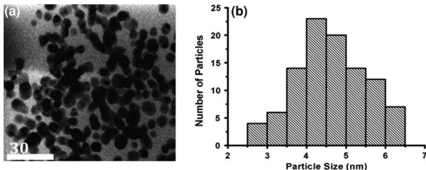
**Fig. 2.5** **a** TEM image of the biogenic silver nanoparticles. **b** Histogram particle size distribution measurements made from the TEM image by counting  $\sim 100$  particles in order to obtain average particle diameter
