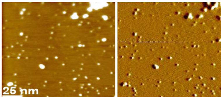
**Fig. 2.6** Atomic force microscopy analysis of the biogenic silver nanoparticles. AFM topographical (*left*) and deflective (*right*) images. The deflection is shown to differentiate single particles and clumps of particles
