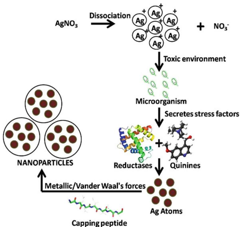
**Fig. 2.1** Schematic mechanism for the biotransformation of metal ions into stable nanocrystallites by microorganisms, illustrated using the biosynthesis of silver nanoparticle by the fungus, *Fusarium oxysporum*
