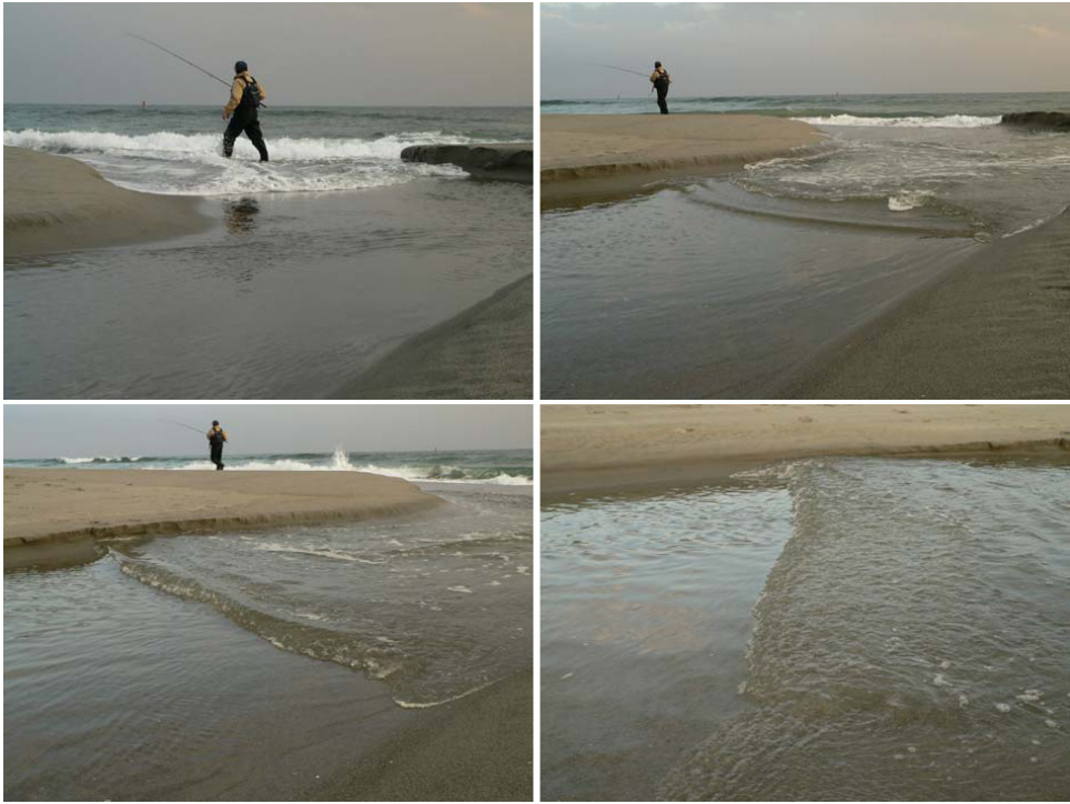
Fig. 1.3. Generation of a bore by the long-wave-induced swash in a freshwater inlet on Takatoyo Beach, Toyohashi (Japan) on 14 November 2008 — Sequence of four photographs: t = t_0 , t = t_0 + 8 s, t = t_0 + 9 s, t = t_0 + 10 s (from left to right, top to bottom).
