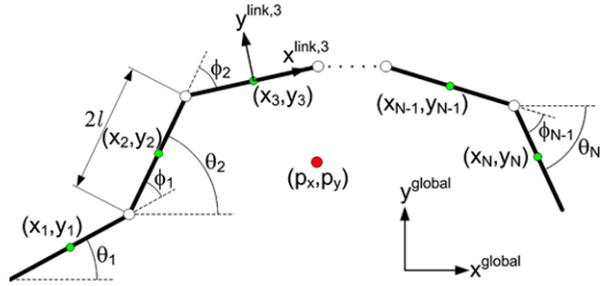
**Fig. 2.2** Forces and torques acting on each link of the snake robot
