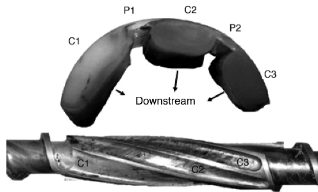
Figure 1.20 A thick frozen section that was cooled and then removed from the screw. For a better understanding of the figure, please refer to the color section.
