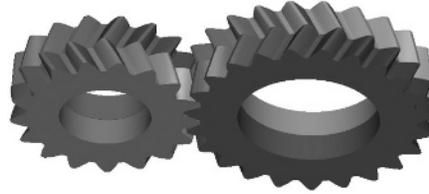
**Figure 1.16** Double spiral or herringbone gears
