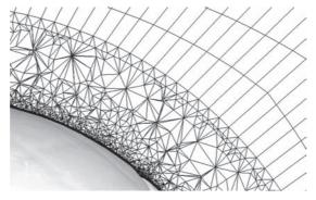
Figure 1.5. An important step in CFD simulations at the University of Sheffield is capturing the geometry of a soccer ball with a three-dimensional noncontact laser scanner. The figure shows part of a soccer ball mesh with approximately 9 million cells. (Courtesy of the University of Sheffield and Ansys UK.)
