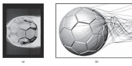
**Figure 1.6.** (a) Wind tunnel smoke test of a nonspinning soccer ball. (b) CFD simulation showing wake-flow path lines of a nonspinning soccer ball, air speed of 27 mph. (Courtesy of the University of Sheffield and Ansys UK.)
