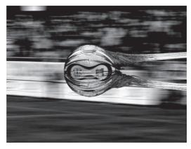
**Figure 1.7.** High-speed airflow path lines colored by local velocity over the 2006 Teamgeist soccer ball. (Courtesy of the University of Sheffield and Ansys UK.)
