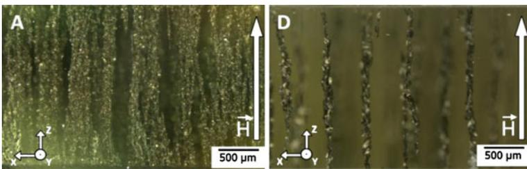
**Fig. 2.9** Micrographs of specimen cross sections with Terfenol-D particles of different size and particle content aligned along magnetic flux lines (*left* particle size  $15 \mu\text{m}$  and 20 wt%; *right* particle size  $< 20$ )
