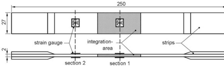
**Fig. 2.4** Specimen design with embedded piezoelectric transducers
