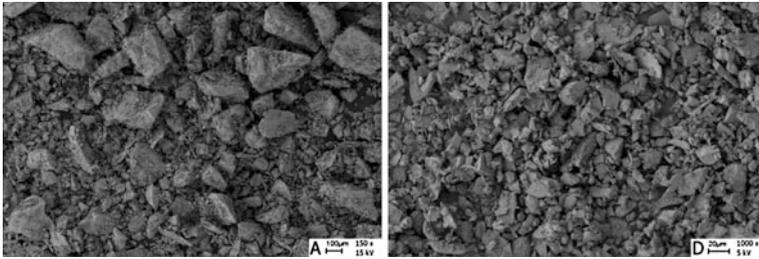
**Fig. 2.8** SEM images of Terfenol particles (*left* original batch; *right* particles after sieving with a size  $< 20 \mu\text{m}$ )
