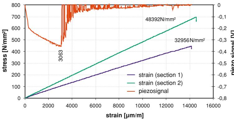
**Fig. 2.5** Exemplary result of a tensile test with a specimen of configuration (b) no cut out
