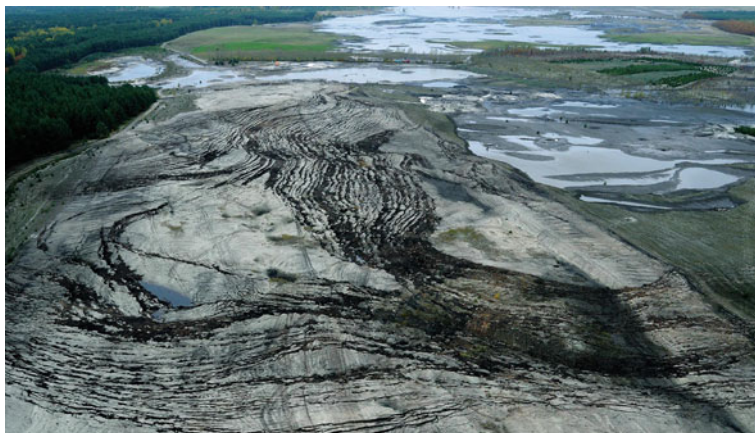
Fig. 2.2 Landslide of dumped overburden in the former Spreetal Mine (Lusatian lignite mining district, Germany) at October 12, 2010. The ground broke over an area of ca. 1800 m × 600 m (ca. 110 ha), damaging the neighbouring pit lake ( upper margin of the photo ). It was caused by an initially local liquidation of deeper parts of the overburden dump and supported by extremely high water saturation of the entire dump as a result of a very rainy period of about 10 weeks. (Photo: Radke, LMBV)
