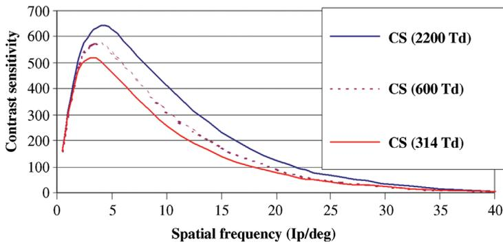
**Figure 1.7** Achromatic contrast sensitivity functions for different values of retinal illuminance level (in Td units). Retinal illuminance corresponds to the luminance
