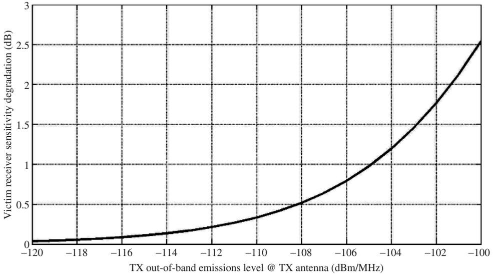
**Figure 1.7** RX sensitivity degradation as a function of the TX out-of-band emissions level by assuming  $-10$  dB coupling factor between the antennas and  $-109$  dBm/MHz receiver noise floor
