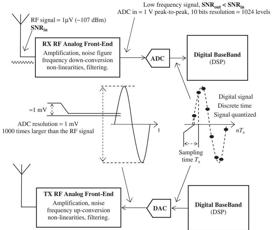
**Figure 1.8** RF analog and DBB partitioning in modern transceivers
