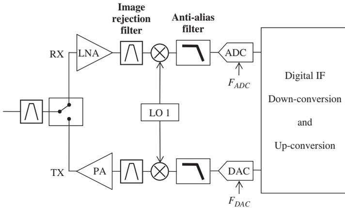
**Figure 1.11** Superheterodyne architecture with digital IF
