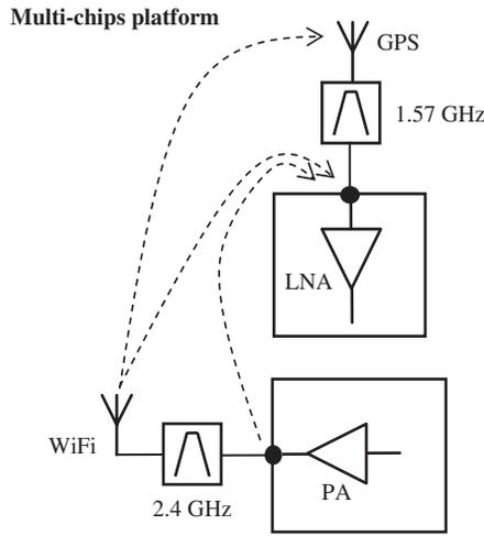
**Figure 1.5** Multi-chips coupling through the antennas
