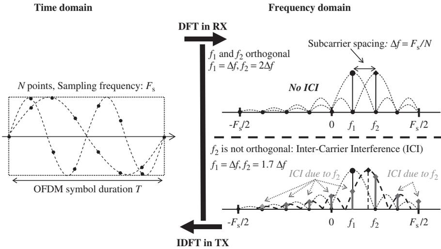
**Figure 1.20** Subcarrier orthogonality and ICI in OFDM
