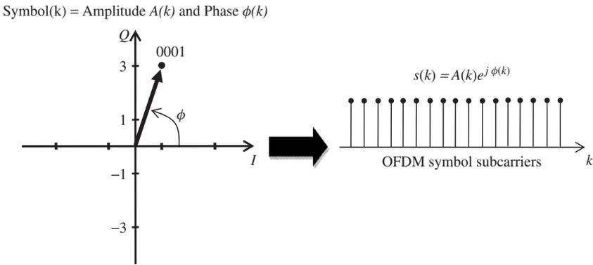
**Figure 1.28** The constellation points determine the amplitude and the phase of the subcarriers
