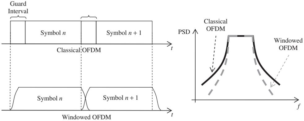
**Figure 1.23** Windowed OFDM reduces the out-of-band emissions of the OFDM transmitter
