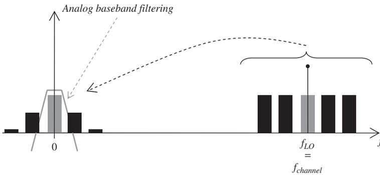
**Figure 1.13** Frequency down-conversion to DC in homodyne or zero-IF architecture
