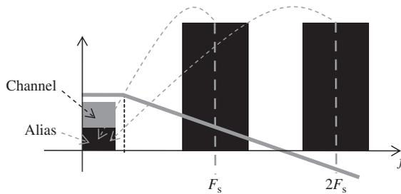
**Figure 1.17** Blockers aliasing before the ADC vs. analog baseband filtering order
