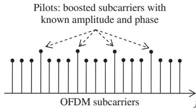
**Figure 1.21** Pilot-tones used in reception for channel estimation
