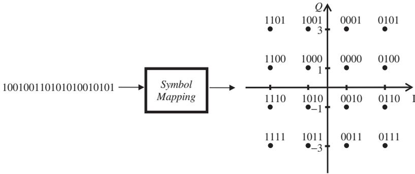
**Figure 1.27** Symbol mapping transforms the bit stream into a complex constellation, here 16-QAM
