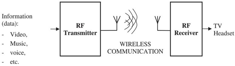
**Figure 1.1** Basic view of an RF communication system
