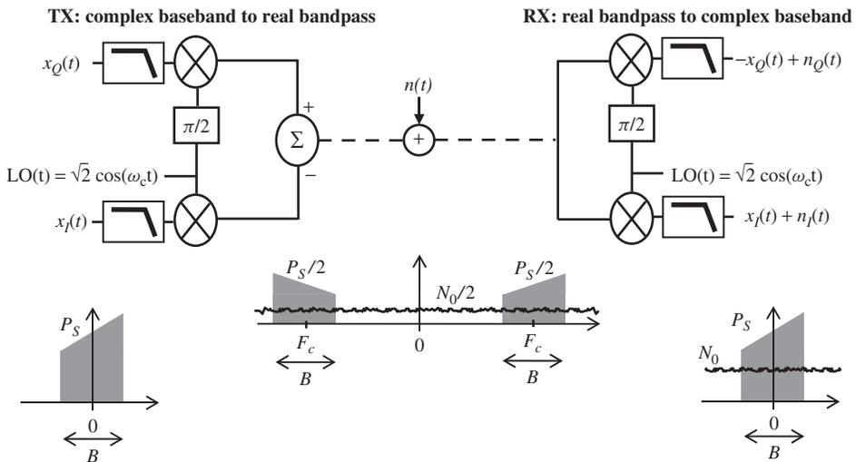
**Figure 1.31** From real bandpass to complex baseband used in system simulations
