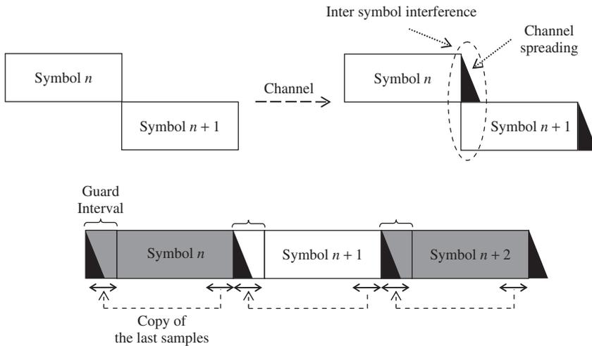
**Figure 1.22** Guard interval insertion in order to combat the channel delay spread and the ISI
