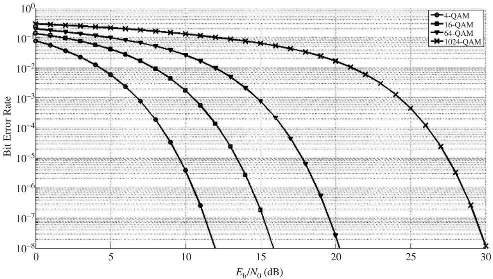
**Figure 1.29** BER vs.  $E_b/N_0$  for 4-QAM, 16-QAM, 64-QAM, and 1024-QAM modulations
