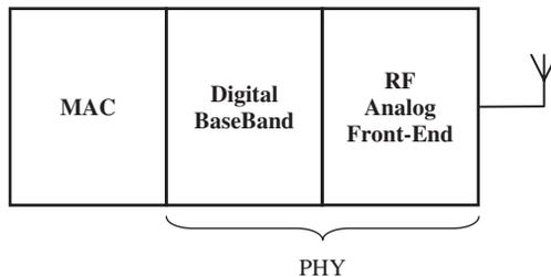
**Figure 1.2** Basic partitioning of a digital communication transceiver
