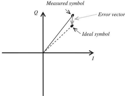
**Figure 1.30** Modulation error vector used for estimating the EVM
