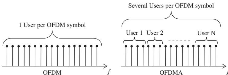
**Figure 1.25** In OFDMA the subcarriers of one OFDM symbol are shared between several users
