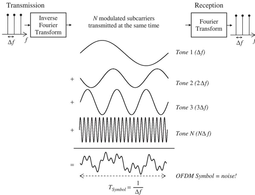
**Figure 1.18** Basic principle of OFDM transmission and reception (baseband illustration)
