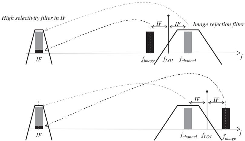
**Figure 1.10** Frequency down-conversion in IF and frequency image issue
