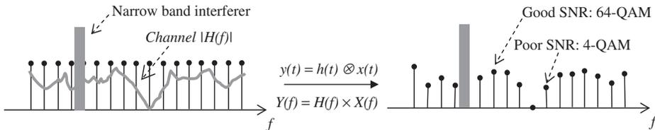
**Figure 1.24** Subcarrier adaptive modulation
