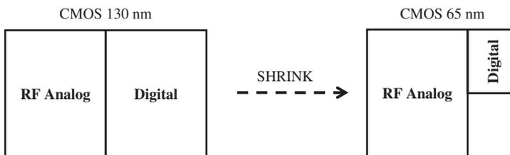
**Figure 1.3** SoC shrink limitation due to the RF analog part of the chip
