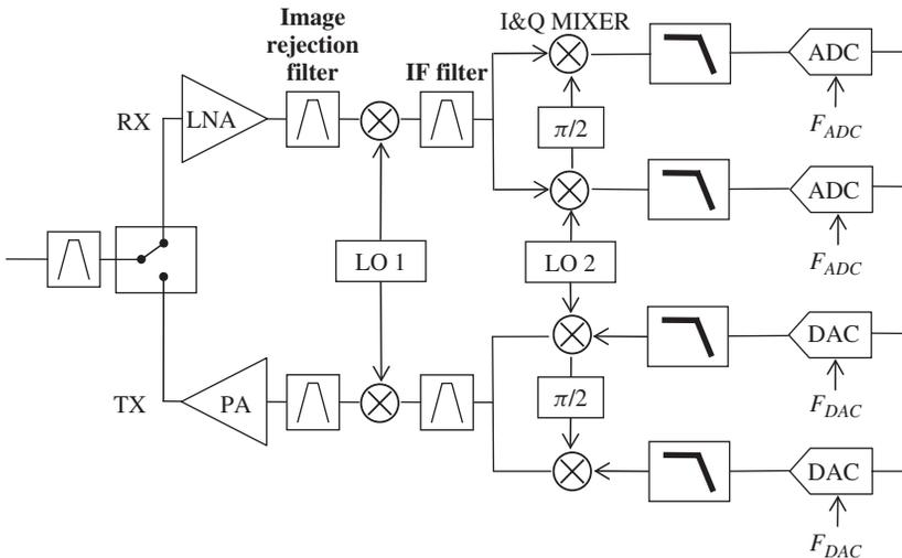
**Figure 1.9** Superheterodyne transceiver
