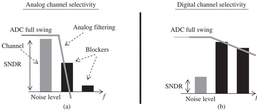
**Figure 1.16** Analog baseband filter order impact on the receiver ADC dynamic range
