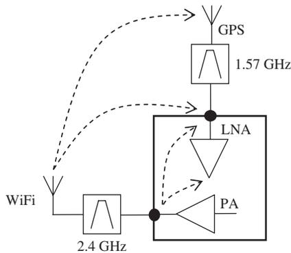
**Figure 1.6** Antennas and systems on-chip coupling
