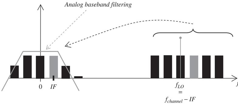
**Figure 1.14** Frequency down-conversion to IF in low-IF architecture
