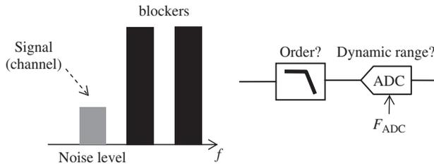
**Figure 1.15** Trade-off between analog baseband filter order and ADC dynamic range
