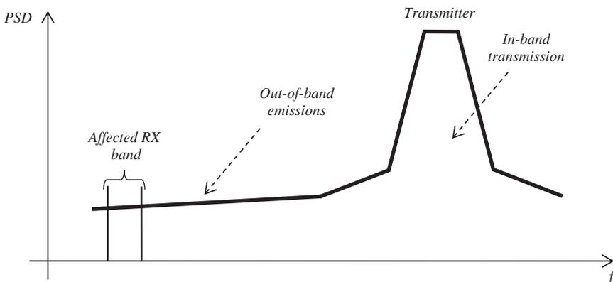
**Figure 1.4** Radio coexistence issues due to transmitter out-of-band emissions
