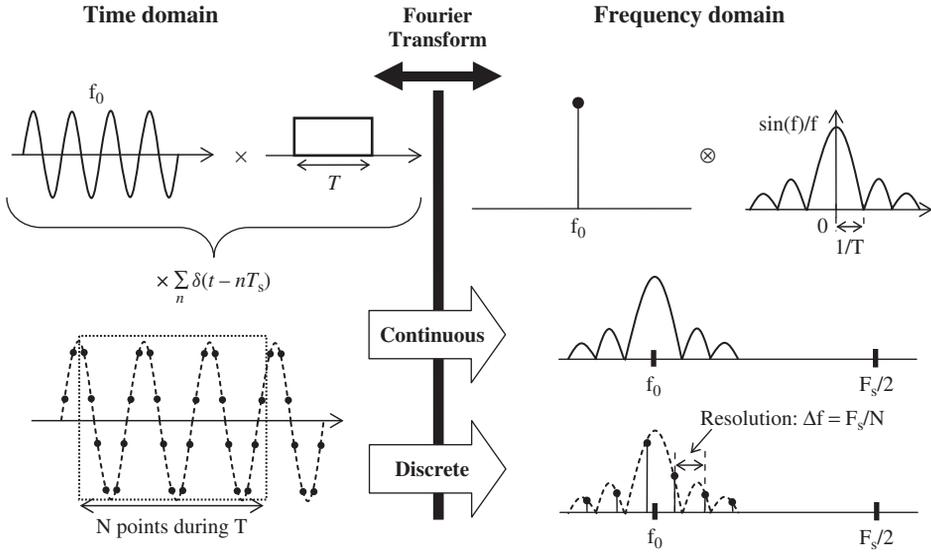
**Figure 1.19** Fourier transform properties important in OFDM
