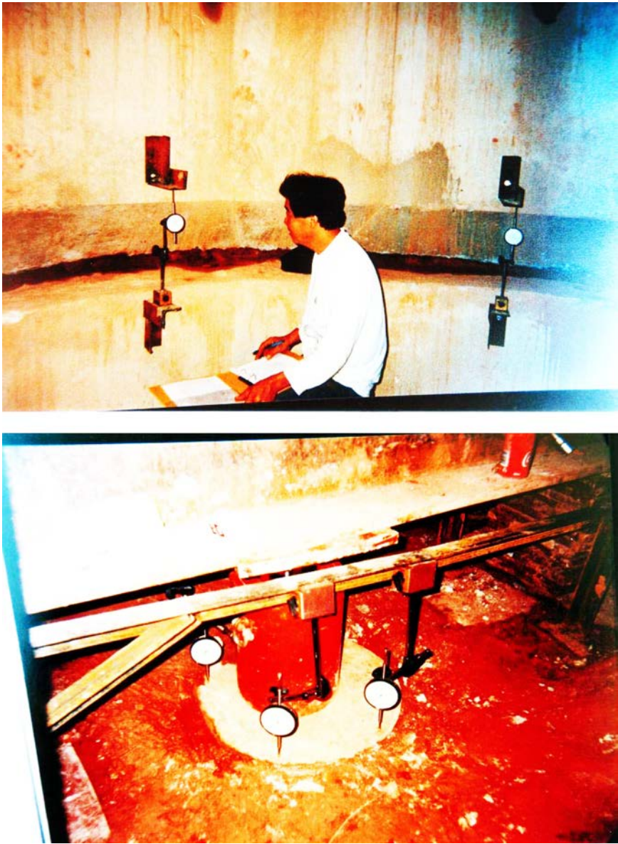
Figure 4.20(b). Monitor displacement using dial gauges.
