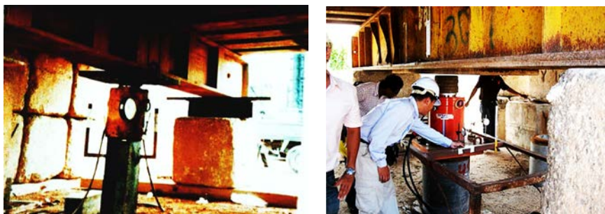
Figure 4.61. Kentledge pile test with a hydraulic jack installed in between the tested pile and the loaded channel. During testing, the hydraulic jack is extended progressively. The applied force versus the displacement of the tested pile is monitored.
