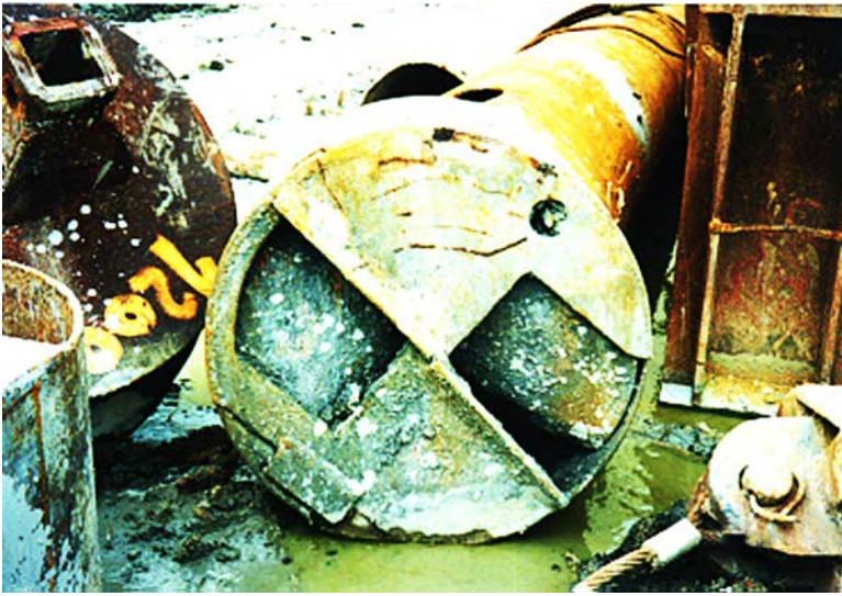
Figure 4.40. A cleaning bucket to clear the crush rocks and flatten the surface at the bottom of a bore hole.
