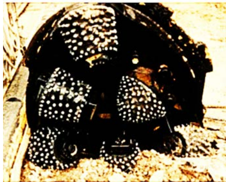
Figure 4.41. Drilling bits of the reverse circulation rig (RCD).
