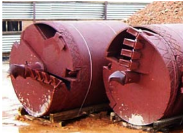
Figure 4.37(a). A boring bucket.
