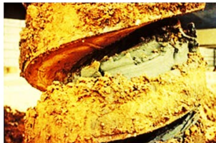
Figure 4.34(b). Augered soil revealing marine clay.
