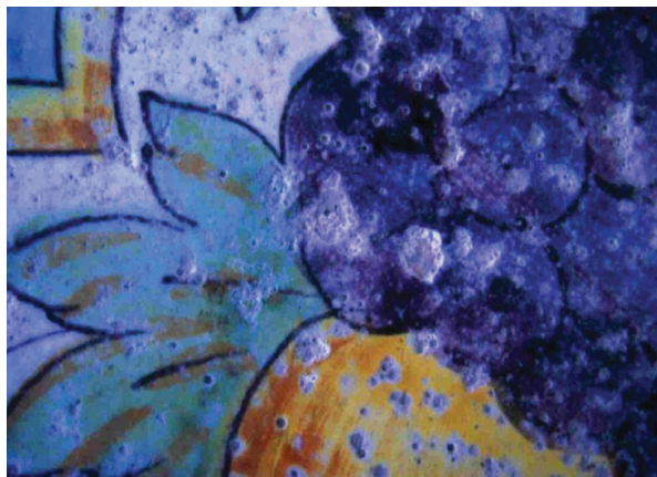
Fig. 1.1 Cracks and pores formed on the surface of a glazed tile (Manises, 18th century) from the floor of the balconies of the Basílica de la Virgen de los Desamparados de Valencia, Spain
