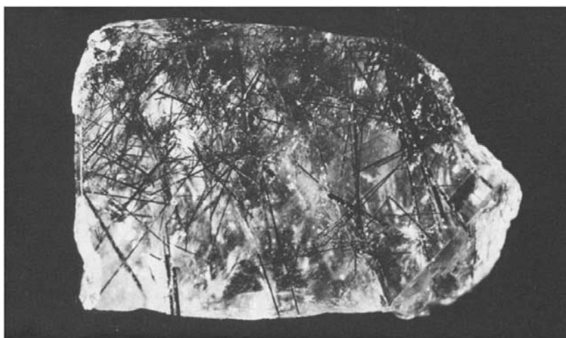
Fig. 1.1.1. Natural growths: needles of (a) tourmaline, and (b) rutile, in quartz.
