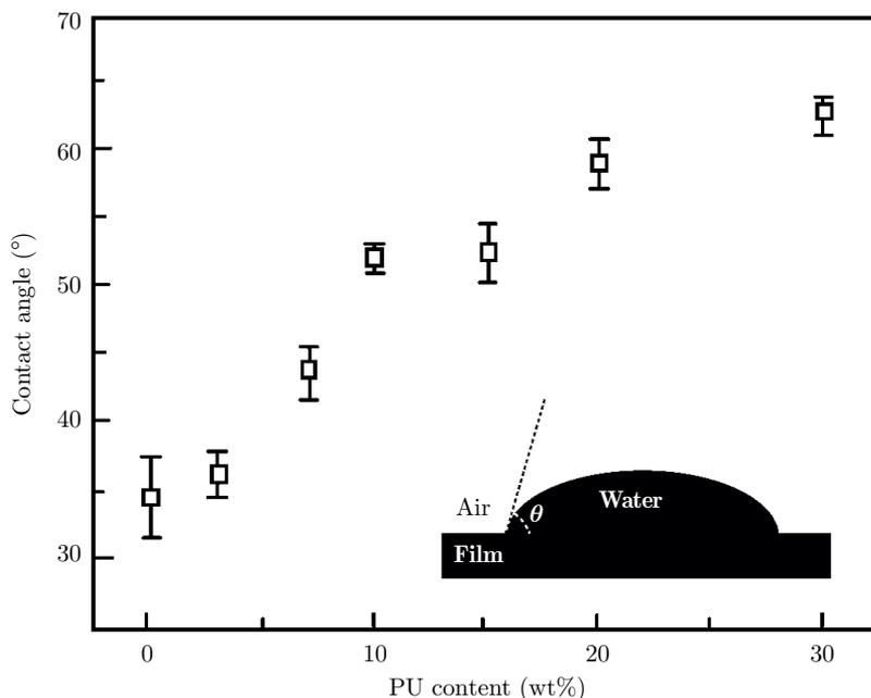
**Figure 5.5.** Contact angle of TPS/PU blends *vs.* PU content [28]
