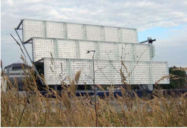
Fig. 2.11. Array of the Ioffe full-size concentrator modules with small aperture area Fresnel lenses
