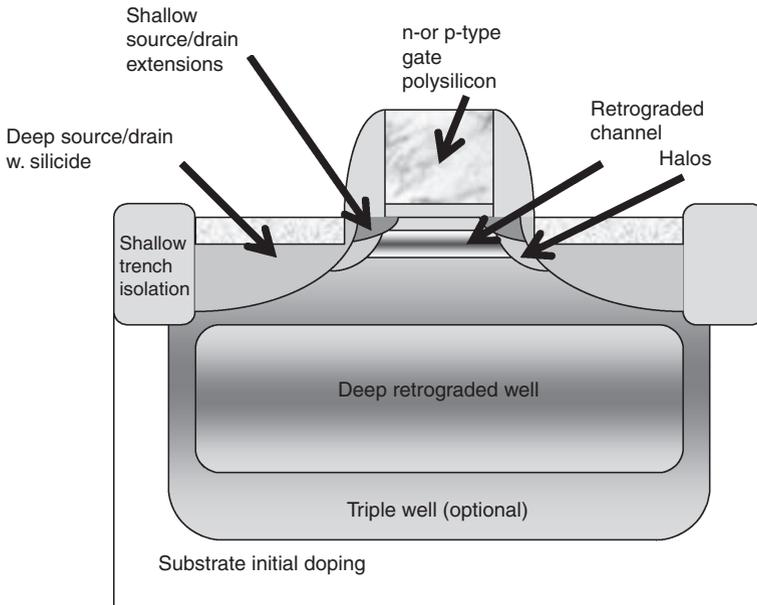
Fig. 3 Overview of the I/I steps needed to fabricate integrated circuits in CMOS technology
