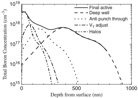
profiles, including the retrograde p-well. The dose variation control of the  $V_T$  adjust is critical for device and circuit applications.
