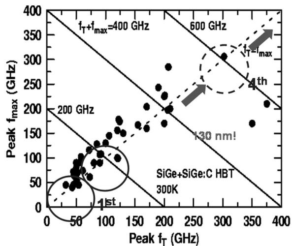
**Fig. 1** Example of SiGe performance evolution over four technology generations. Courtesy of John D. Cressler, Institute of Technology, Atlanta, GA [5]
