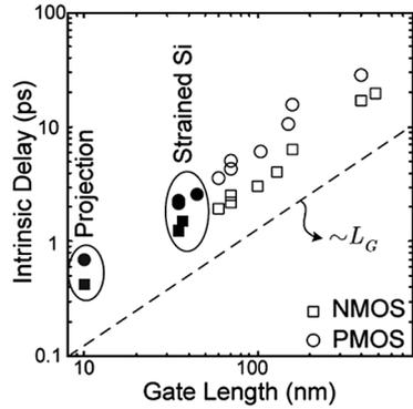
a very important concept to keep CMOS on the roadmap [9]. Figure 2 illustrates how strain induced mobility enhancement was introduced at about the 90 nm technology node (see the next section for a definition), to ensure continued performance scaling for shorter gate lengths.
