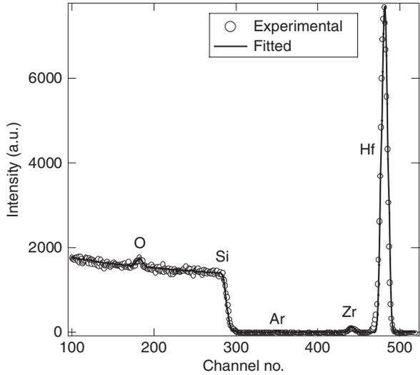
Structure and Nanoscale Depth Profiling” *medium energy ion scattering* and *time of flight-energy elastic recoil detection analysis* (ToF-E ERDA) will be discussed. Another commonly used technique is *Rutherford Back Scattering* (RBS). RBS is an important analysis tool for thin films in microelectronics. The composition of Hf-based films can be determined with resolution below the percent level; an example is shown in Fig. 7 [24].
