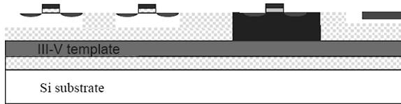
**Fig. 10** Cross section of a future silicon wafer with integrated areas of III-V devices. Courtesy of E. Fitzgerald, Massachusetts Institute of Technology, Cambridge
