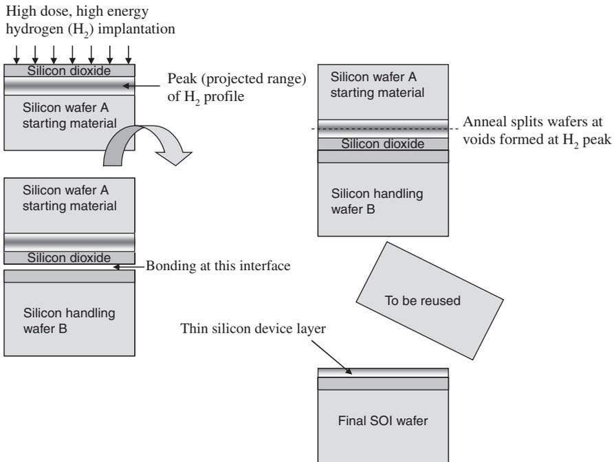
**Fig. 8** Example of hydrogen implantation to form an SOI substrate with a buried oxide layer [16, 25]
