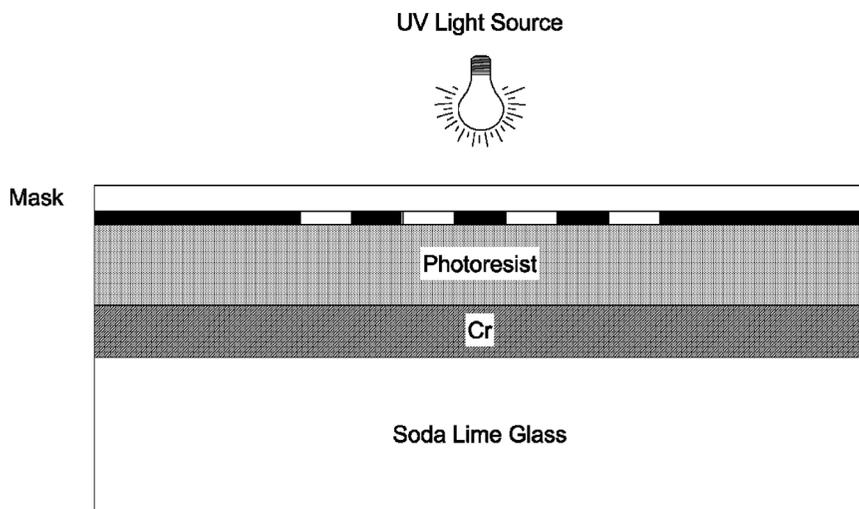
Fig. 4. Schematic of bottom substrate photoresist layer upon exposure to ultraviolet light.
