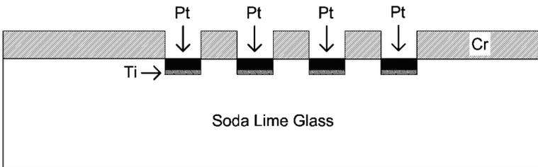
Fig. 10. Schematic of bottom substrate after lift-off process.
