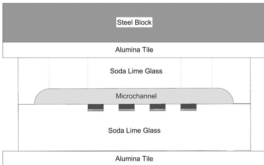
Fig. 19. Schematic of bonding “stack” prior to insertion in furnace for thermal bonding.
