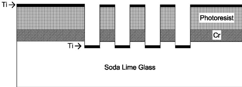
Fig. 8. Schematic of Ti deposited layer.
