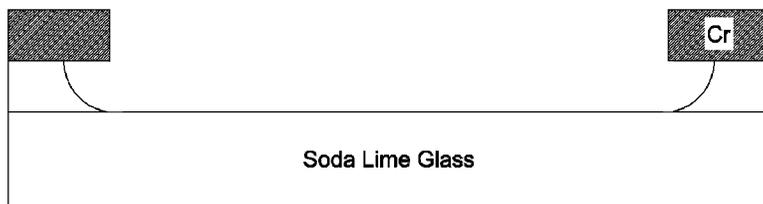
Fig. 16. Schematic of top substrate following glass etching.
