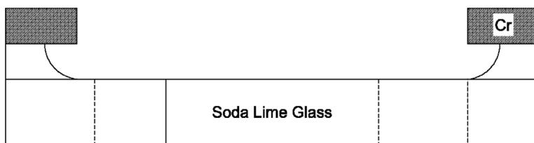
Fig. 17. Schematic of top substrate following reservoir drilling.
