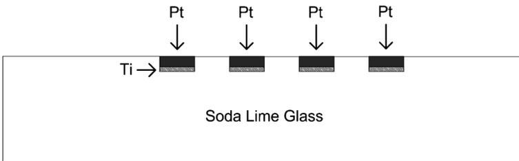
Fig. 11. Schematic of completed bottom substrate with recessed electrodes.
