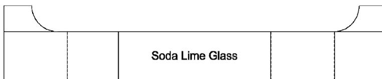
Fig. 18. Schematic of top substrate following removal of the chrome layer.
