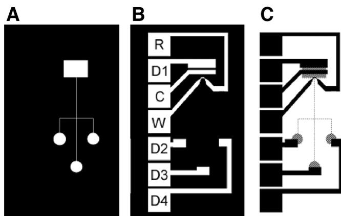
the location of the larger reservoir required to accommodate the EC detection and CE driving electrodes. In **Fig. 2B**, R = the reference electrode; C = the counter electrode; W = the working/detection electrode; and D1, D2, D3, and D4 are the driving electrodes for the detection, sample, buffer, and waste reservoirs, respectively.
