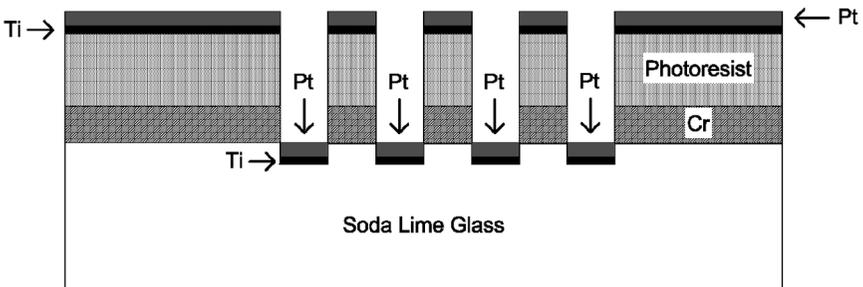
Fig. 9. Schematic of Pt deposited layer.
