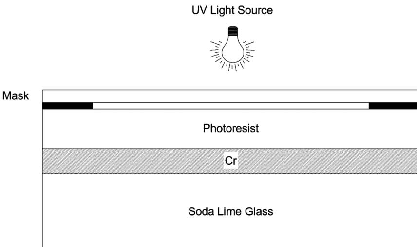
Fig. 12. Schematic of top substrate patterning with ultraviolet light.
