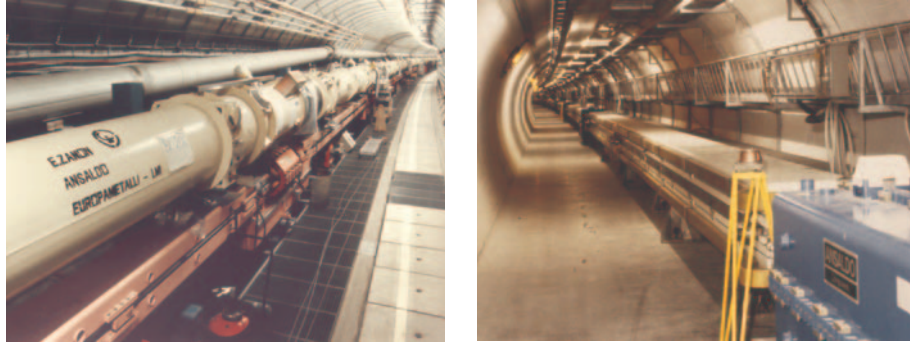
Figure 1.3 Left: High Energy Ring Accelerator (HERA) at DESY [33], Hamburg, Germany, where in one ring the normal-conducting magnets steer the electron beam and in the other the superconducting magnets steer the counter-rotating proton beam. Right: LEP quadrupole and dipoles. The main dipoles have a bending field of 0.109 T at a beam energy of 100 GeV.
