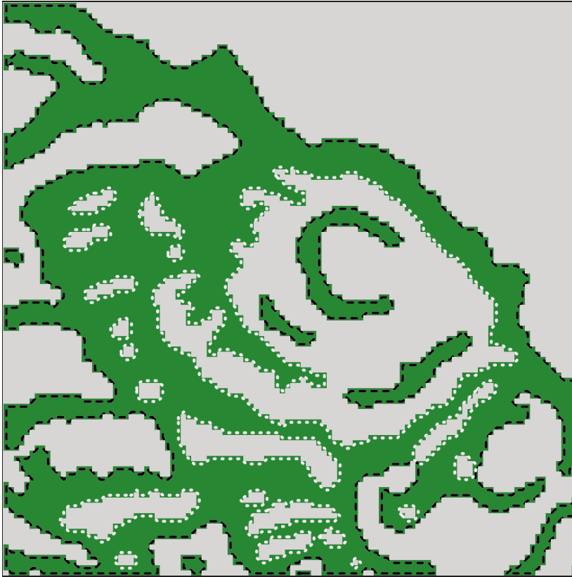
Figure 2.11 Example of a complex contour (in a section cut from Fig. 7.12 in Vol. 1 [14]). Outer contours are marked in black and inner contours in white.
