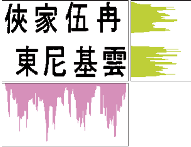
Figure 2.20 Example of the horizontal projection P_{\text{hor}}(v) (right) and vertical projection P_{\text{ver}}(u) (bottom) of a binary image.
