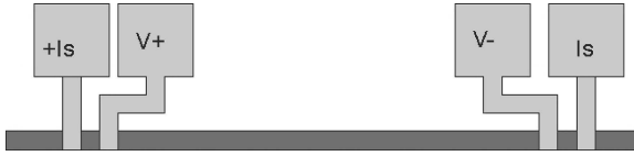
Fig. 8 Kelvin connected magnetoresistor
