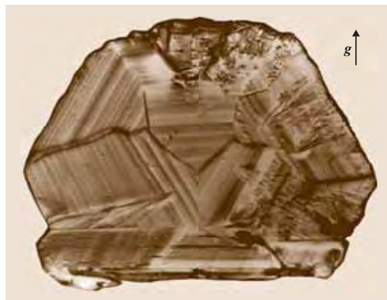
Fig. 4.9 X-ray topograph of a (0001) plate (about 8 mm diameter, 0.35 mm thick) cut out of a quartz-homeotypic gallium phosphate \text{GaPO}_4 crystal grown from high-temperature solution in phosphoric/sulphuric acid [4.47]. It shows the triangular arrangement of growth sectors with pronounced striations. Growth-sector boundaries are visible by topographic contrast or by the bends of the striations. Diffraction vector g(10\bar{1}0) , \text{AgK}\alpha radiation
