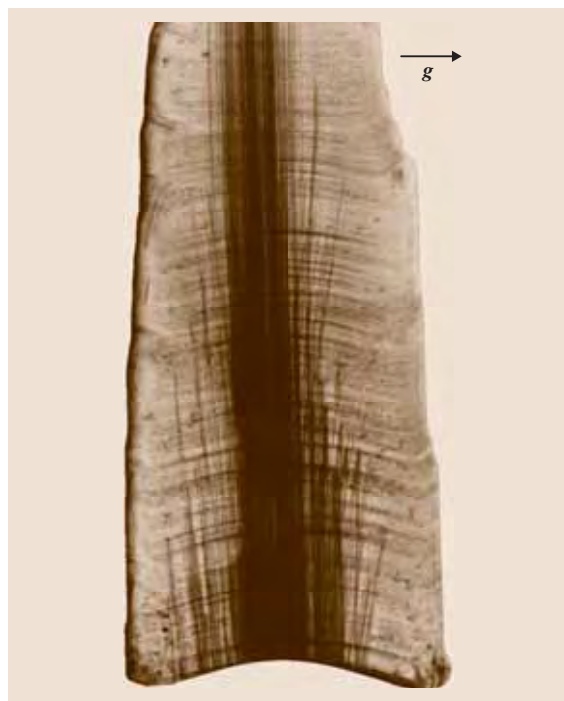
Fig. 4.10 Plate cut from the center of a Czochralski boule of orthorhombic salol ( T_m = 42^\circ\text{C} ), about 1.3 mm thick, imaged length about 40 mm. The growth striations marking the interface at different stages of growth contain tiny gas bubbles, many of which are sources of growth dislocations. Due to the concave interface the dislocations are focussed toward the center of the boule. Due to this effect many dislocations enter the plate from above through the plate surface. Diffraction vector g(002) , \text{CuK}\alpha_1 radiation
