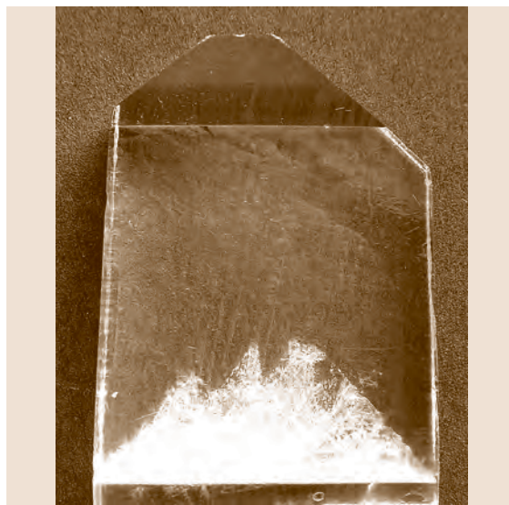
Fig. 4.2 A KDP crystal (length 45 mm) with {011} capping pyramid on a {001} seed plate
