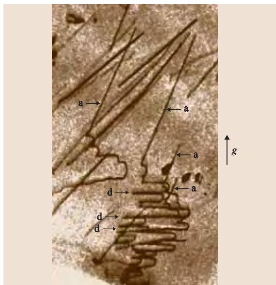
Fig. 4.25 Section (about 4 \times 7 \text{ mm}^2 ) of a (110) plate (about 1.5 mm thick) of benzophenone grown from supercooled melt. The large arrows mark four growth dislocation in a (111) sector showing sharply defined non-crystallographic preferred directions (predominantly screw character) in their upper, and post-growth movement with pinning stops in their lower parts. Burgers vector b = [001] vertical. The horizontal segments are pure-edge and form a few dislocation dipoles (small arrows). The dislocations emerge through the plate surfaces. g(002) , \text{CuK}\alpha_1
