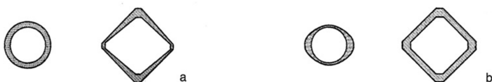
Fig. 6.11 Ovalized tooling promotes wall thickness uniformity: (a) standard round tooling and (b) ovalized die tooling
