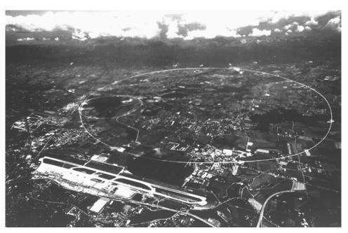
Fig. 1.3. An aerial view of CERN-Geneva, showing the undeground LEP ring, 27 km in circumference, where also the LHC (large hadron collider) will run soon. In order to see the real size of the ring, one can see Geneva airport in the front part of the photo (ref. CERN X 973-1-87).
