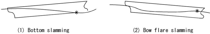
**Fig. 2.2.3** Types of slamming impact of a ship
