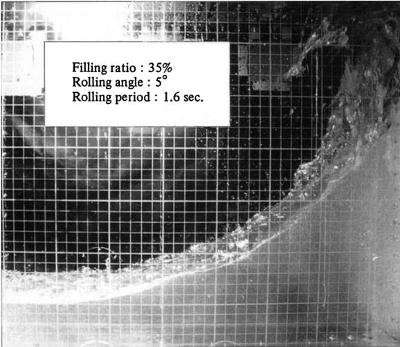
Fig. 2.3.3 Sloshing test of a rectangular tank
