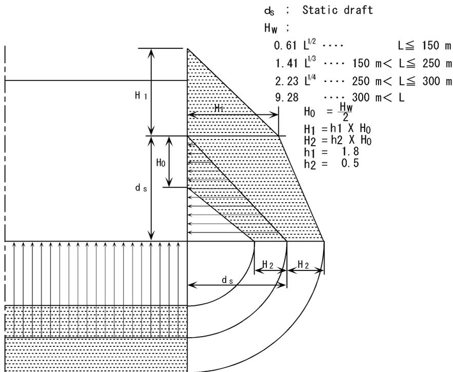
Fig. 2.3.1 Transverse strength calculation loads by NK
