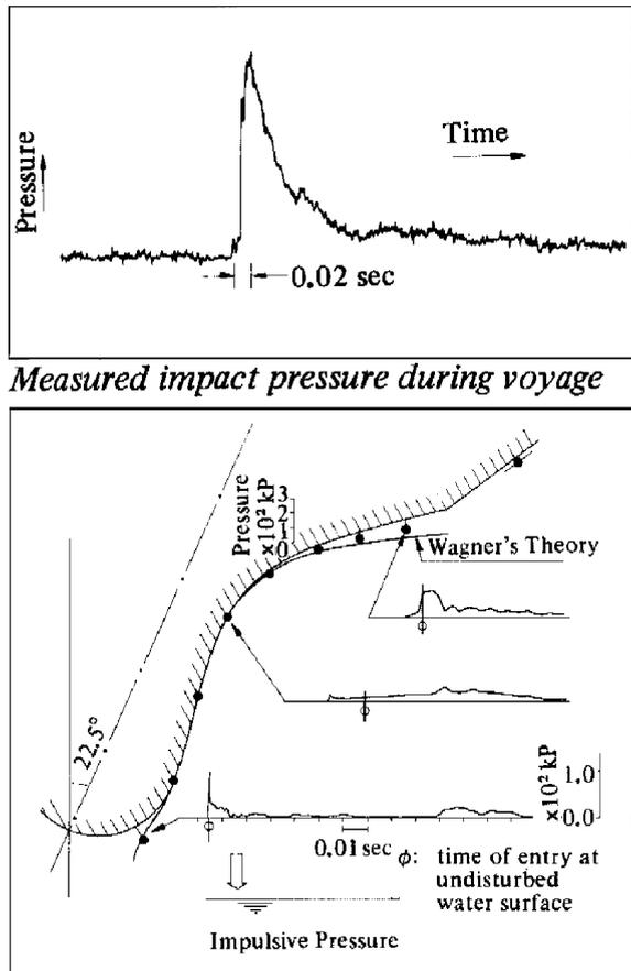
Fig. 2.3.2 Drop test results of inclined 2- dim. model
