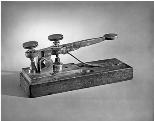
Figure 1.1 The original telegraph key used by Samuel F.B. Morse in 1844 (reproduced with permission of the Smithsonian Institution).
