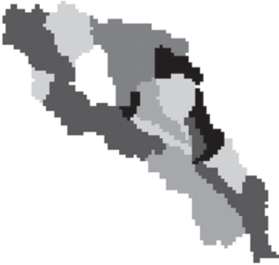
FIGURE 1.3. Raster cell-based approach versus lumped patch or polygon-based approach. The higher complexity of the cell-based approach adds flexibility and versatility to the simulations.
