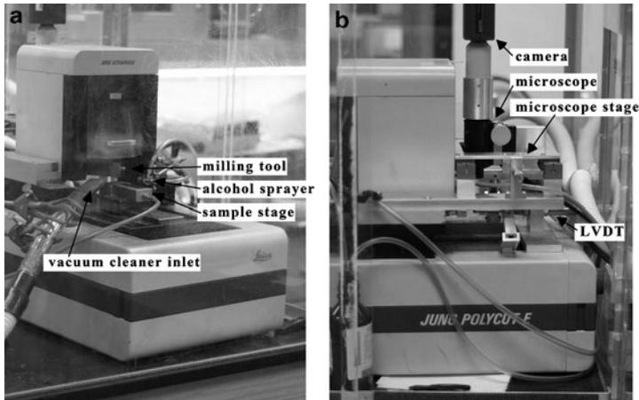
**Fig. 3** The automated serial sectioning device developed by Alkemper and Voorhees (Alkemper and Voorhees 2001). (a) Image of the commercial Reichert-Jung Polycut E micromiller system, with modifications by A&V for cleaning the sample after the micromilling operation. (b) View of the microscope attachment and LVDT installed by A&V to perform automated serial sectioning. Figure is adapted from (Alkemper and Voorhees 2001) with permission from Wiley
