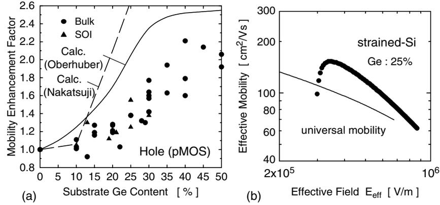
**Fig. 1.6.** Mobility characteristics of bi-axial tensile strained Si p-channel MOSFETs (a) Mobility enhancement factor as a function of Ge content in SiGe substrates. Symbols show experimental results. Closed circles and triangles show the values in bulk and SOI MOSFETs, respectively. Solid [46] and dash [47] lines mean the results of theoretical calculations. (b)  $E_{\text{eff}}$  dependence of hole mobility in bi-axial tensile-strain Si p-channel MOSFETs
