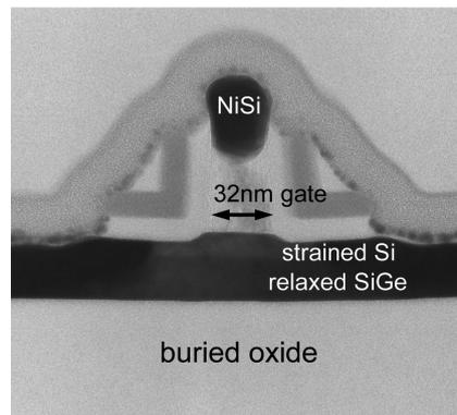
**Fig. 1.10.** TEM photograph of cross-sectional view of a strained Si-On-Insulator MOSFET with gate length of 32 nm [31]. A strained-Si thin film, where a channel of the MOSFET is formed, and a relaxed-SiGe thin film are fabricated on a buried oxide layer. The gate electrode is made of poly-Si and NiSi formed in source/drain region and on the top of the poly-Si gate
