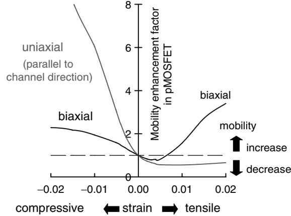
**Fig. 1.8.** Calculated results of the mobility enhancement factor for inversion-layer holes in Si p-channel MOSFETs with uni-axial compressive and bi-axial tensile strain [38]. The value of  $E_{\text{eff}}$  is taken to be  $1 \text{ MV cm}^{-1}$
