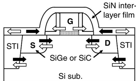
**Fig. 1.11.** Schematic illustration of a device structure using a variety of local strain techniques. STI in the figure means regions of Shallow Trench Isolation. *Black and white* arrows indicate compressive and tensile strain, respectively
