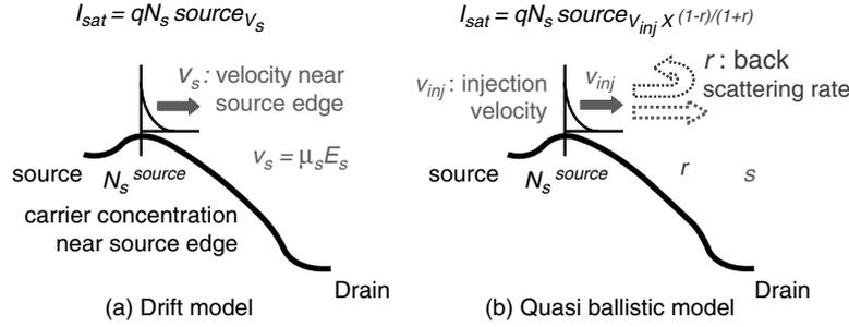
**Fig. 1.1.** Schematic diagrams to show factors to dominate current drive,  $I_{sat}$ . Fig. 1.1(a) and (b) show the diagrams based on a classical drift model and a quasi-ballistic model, respectively.  $E_s$ ,  $q$  and  $\mu_s$  mean the lateral electric field, the elementary charge and mobility near source region, respectively
