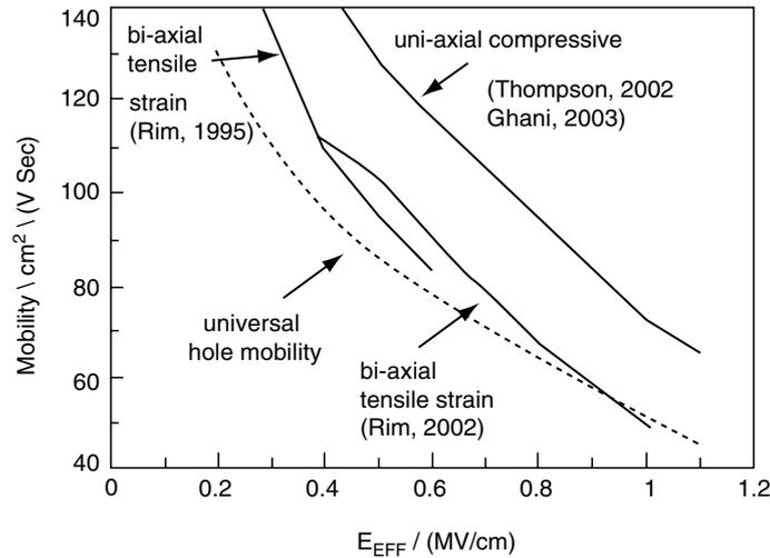
**Fig. 1.7.** Experimental results of the  $E_{\text{eff}}$  dependence of hole mobility in Si p-channel MOSFETs with uni-axial compressive and bi-axial tensile strain
