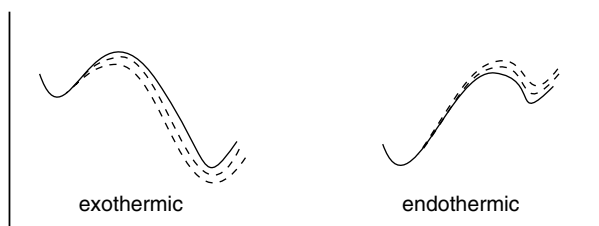
Fig. 3.9. Energy profiles for series of related reactions illustrating the Bell-Evans-Polyani relationship.
