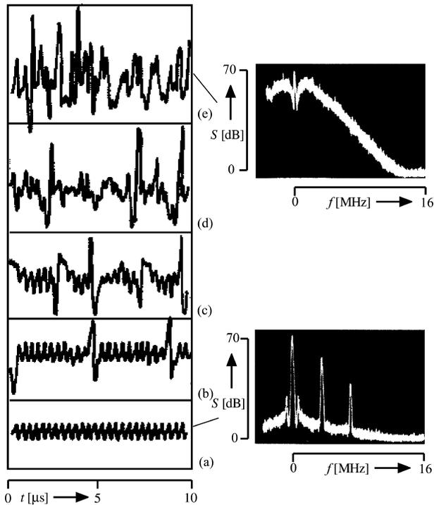
**Fig. 2.2.** Experimentally observed chaotic time series in an infrared He-Ne laser. Stable oscillation state (a) to chaotic state e. One of the mirrors in the laser cavity is tilted and the bad-cavity condition is realized (after Weiss CO, Godone A, Olafsson A (1983); © 1983 APS)
