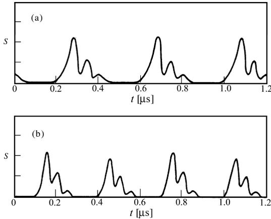
**Fig. 2.4.** Experimental plots of pulsation instabilities in an Xe laser at  $3.51\ \mu\text{m}$  oscillation for **a** period-1 pulsation at a discharge current of 40 mA and **b** period-2 pulsations at a discharge current of 50 mA (after Casperson LW (1978); © 1978 IEEE)
