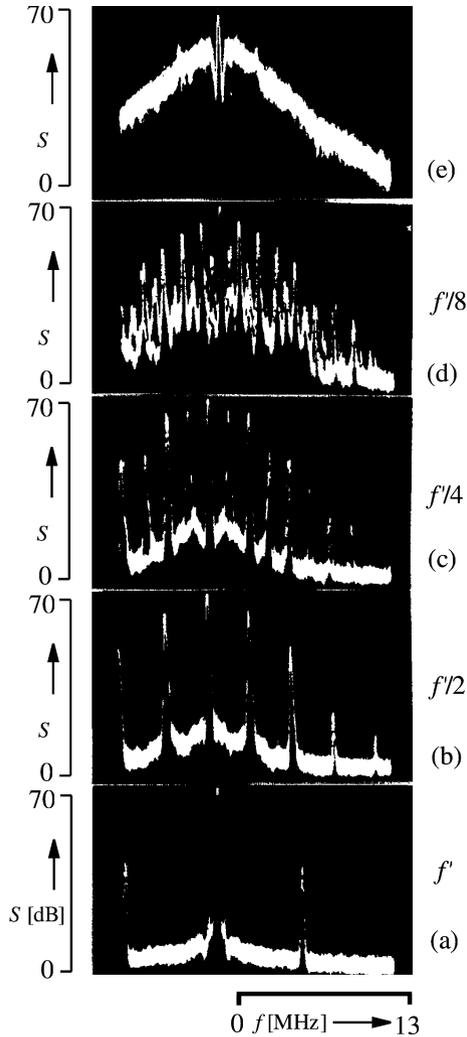
**Fig. 2.3.** Experimentally observed optical power spectra in an infrared He-Ne laser for period-doubling route to chaos. Tilting of one of the resonator mirrors leads to oscillations to **a** period-1, **b** period-2, **c** period-4, **d** period-8, and **e** chaos (after Weiss CO, Godone A, Olafsson A (1983); © 1983 APS)
