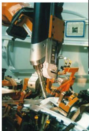
Fig. 22 Laser-MIG-hybrid welding, industrial application, lightweight aluminium car door, VW phaeton
