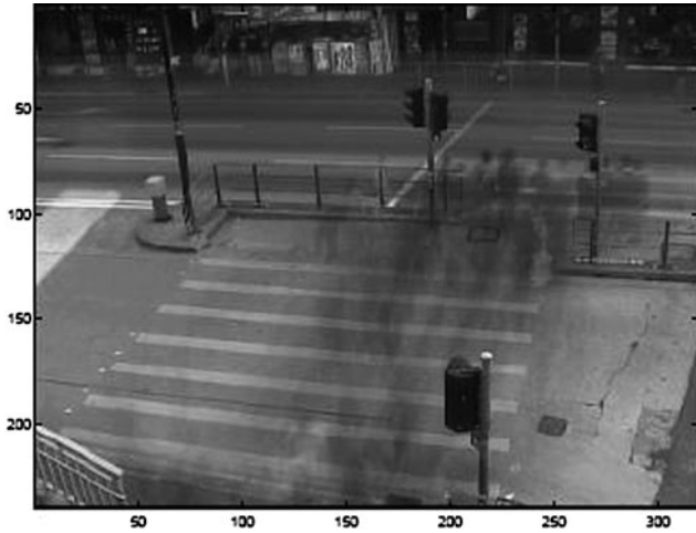
Fig. 2.2 The Result Background of Multi-frame Average Method
