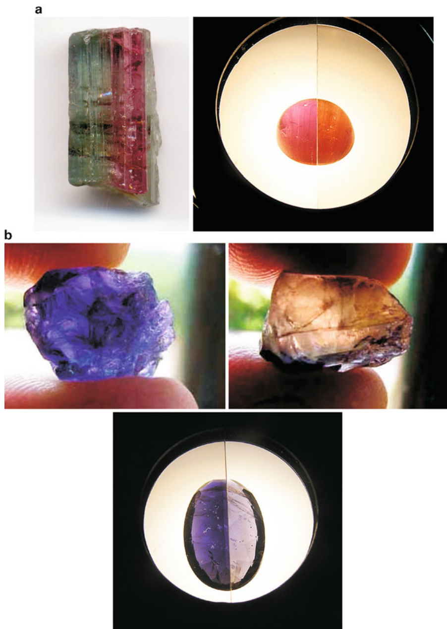
Figure 2.66. Dichroscope images of (a) dichroism exhibited by tourmaline; (b) trichroism exhibited by iolite. Images taken from http://www.nordskip.com/pleochroism.html . [56]
