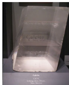
Figure 2.65. Illustration of the double refraction phenomenon exhibited by calcite crystals.
