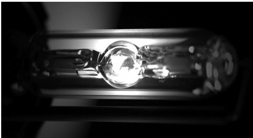
Fig. 2.1 High temperature Xenon lamp made from high purity quartz
