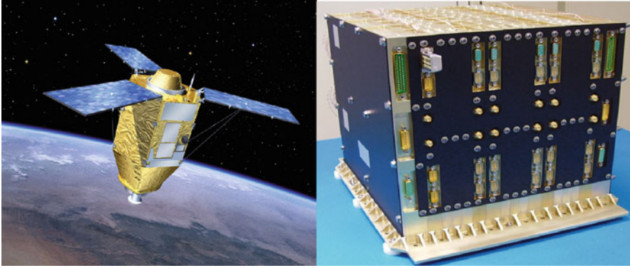
Fig. 2.6 PLEIADES-HR satellite and its compression unit
