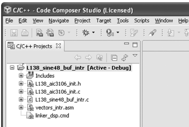
Figure 1.22 Project View window after linking support files to project L138_sine48_buf_intr .
