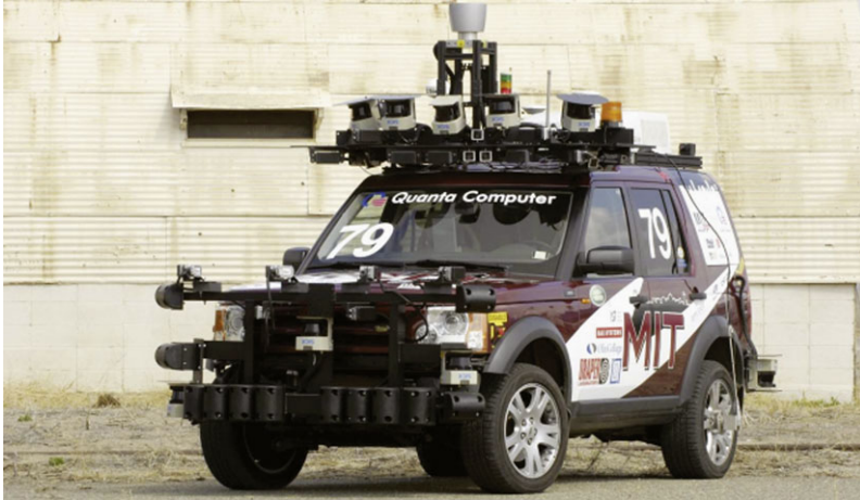
Fig. 2.4 The intelligent vehicle Talos developed by the Team MIT (published courtesy of Massachusetts Institute of Technology)
