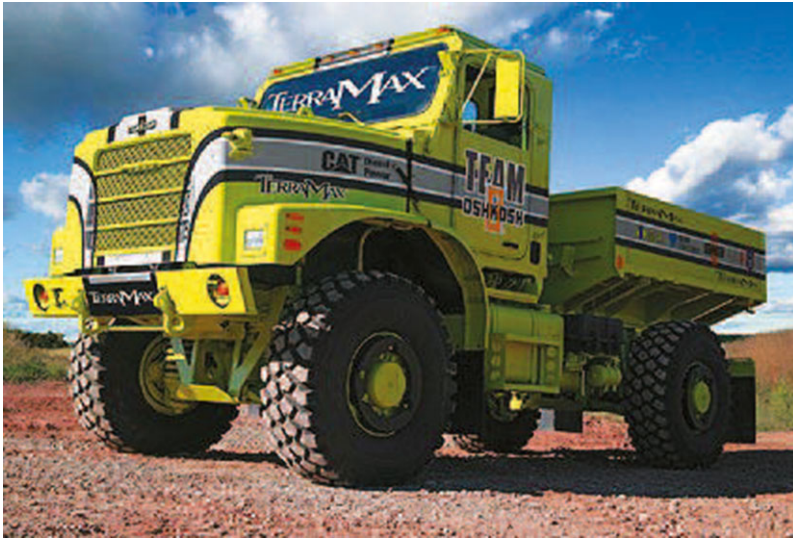
Fig. 2.7 The intelligent vehicle TerraMax (published courtesy of the Oshkosh Truck Corporation)
