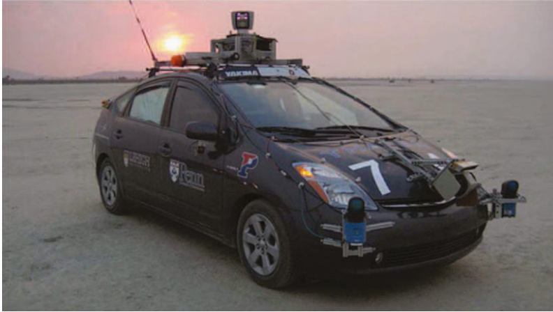
Fig. 2.6 The intelligent vehicle Little Ben (published courtesy of the University of Pennsylvania and Lehigh University)
