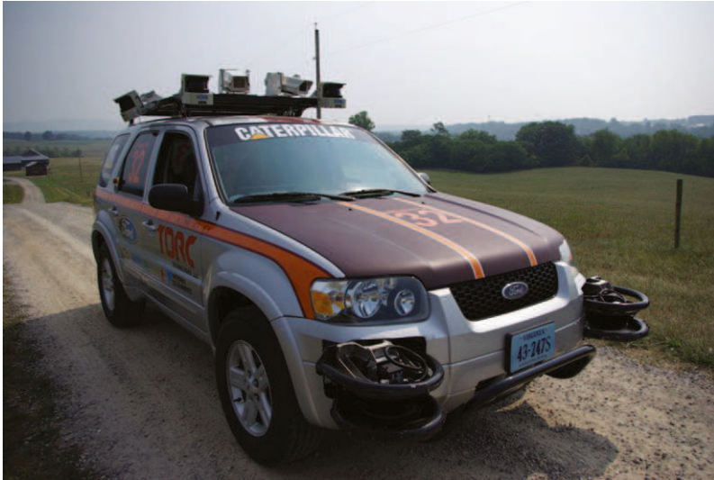
Fig. 2.3 The intelligent vehicle Odin developed by the Team VictorTango (published courtesy of Virginia Polytechnic Institute and State University)
